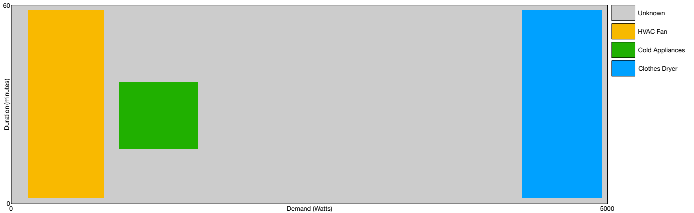
Fig. 5. An example of a coloured partition map to auto-label North American appliances. Each country/region would have their own specific partition map based on readily available appliance statistics for government organizations and manufacturers. Using \mathbf{P}[d, p, r] , and example where the duration is 30min, the power demand is 4.5kW, and the region is North America (NA); \mathbf{P}[30, 4500, \text{'NA'}] would return the colour “blue”, which is associated with the appliance label “Clothes Dryer”.
